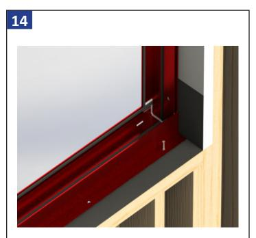
Center and set the flashing flange system into the rough opening. Pulling the system tight towards the interior making sure flashing flange is tight against the WRB. Temporarily screw the window into place using a screw through the pre-drilled pilot holes on the sub-sill anchor flange. **Do not** screw through flashing flange.
