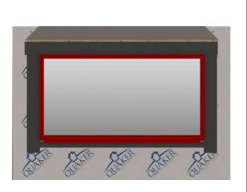
Cut a piece of flashing tape for the head flashing, which extends beyond outer edges of jamb flashings. Remove release paper and install completely covering mounting flange and adhering to exposed sheathing or framing members.
