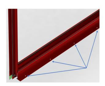
Test fit the flashing flange system into the opening to ensure a proper fit that is plumb, level, and square. Check and mark points in sub-sill anchor flange, jamb & head receptors for places to drill pilot holes for installation. Remove flashing flange system.
