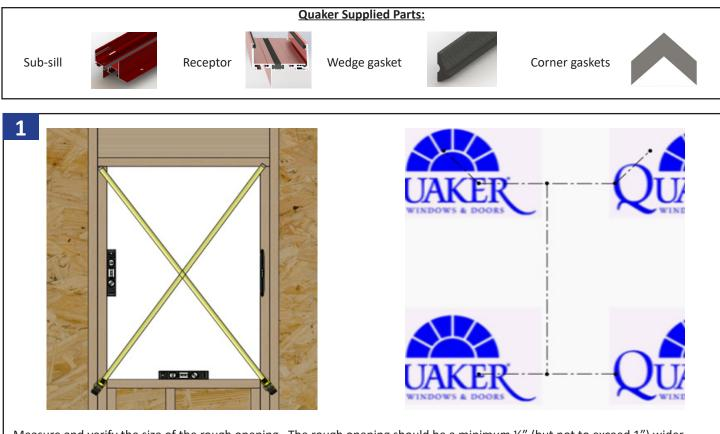
Measure and verify the size of the rough opening. The rough opening should be a minimum ½" (but not to exceed 1") wider and taller than your flanged sub-sill/receptor unit. Verify the rough opening is flat, plumb, level, and square. Take diagonal measurements to check for square. The sill plate beneath the unit must be level for proper unit operation. Cut the weather-resistant barrier (WRB) in a "I" pattern. Cut the top corners of the WRB at 135° and 9" long.
