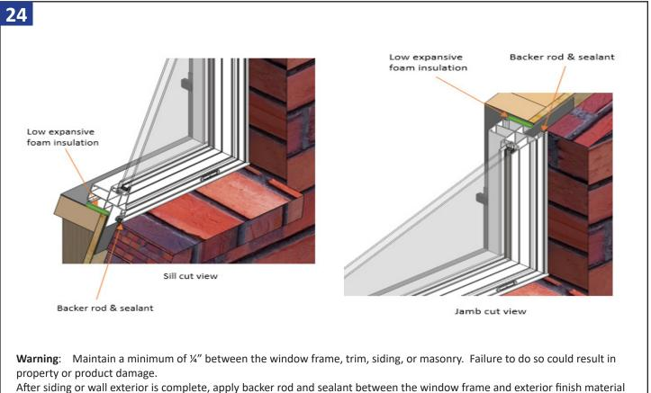
After siding or wall exterior is complete, apply backer rod and sealant between the window frame and exterior finish mat on all four sides of unit. Make sure to clean all surfaces before applying sealant.
