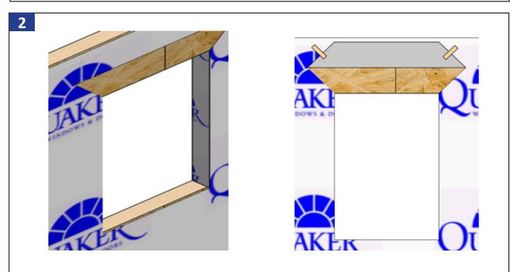
Fold back the WRB sides and sill toward the interior and staple into place. Fold flap up and temporarily tape in place as shown above.
