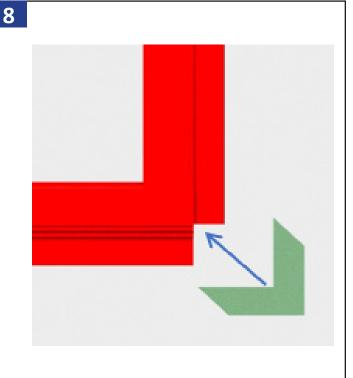
Peel backing off the supplied corner gaskets and install over exterior side of flashing flange on the bottom two corners to cover gap between flanges.
