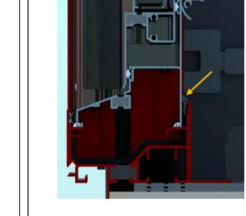
Place a level on the window sill to verify that the sill is level. Adjust the shims as needed to ensure a level condition. Apply the sub-sill wedge gasket into the interior side of the sub-sill against the window.
