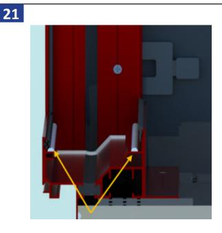
Apply a bead of sealant to the legs of the sub-sill where the window will rest.
