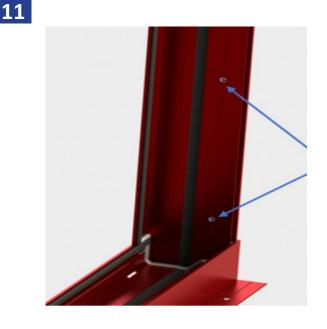
Drill pilot holes in the jamb and head receptor per shop drawings or anchorage calculations. Typically 3" from the corners and 12" on center. Keep all pilot holes on the interior side of flashing flange.
