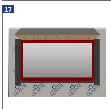
Cut two pieces of flashing tape for jamb flashing extending 1" above flashing flange system head flange and 4" to 6" below bottom edge of sill flashing. Remove release paper and press tightly along sides of window frame.
